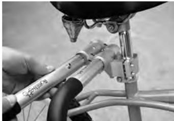
8. Align the spline features and slide the bars into the mounted tubes until the push-button clicks into place.
