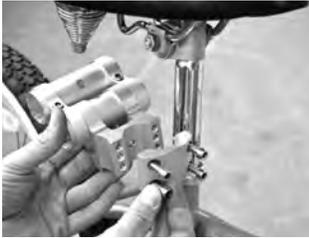
1. Loosen and remove the four 5mm bolts on the seatpost clamp.
