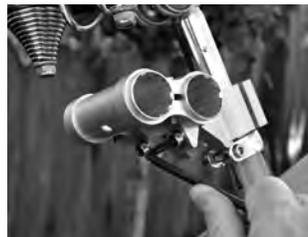
5. Use the rear facing mounted tube bolts to adjust the angle of the mounted tube closest to the seat post.
