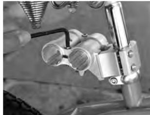
6. Use the twin tube clamp bolts to adjust the angle of the twin tube clamp itself as well as the rear mounted tube.
