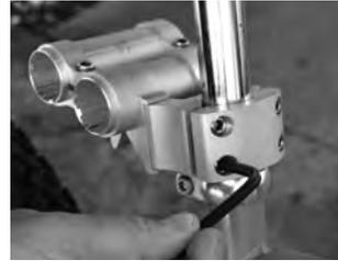
3. Place the clamp around the post and reinstall/tighten the bolts.
