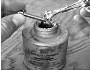
2. We recommend applying anti-sieze or grease to all bolt threads.
