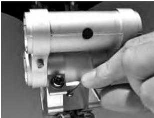
4. Tighten the set screw on the back of the clamp to further prevent rotation of the mount on your post.
